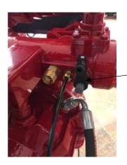
The pressure sensor, which can be adjusted in the range of 0.5-2 bar, sends signals to the solenoid valve and clutch once the system reaches the desired pressure. As a result of the signal it sends, the vacuum is disabled.
